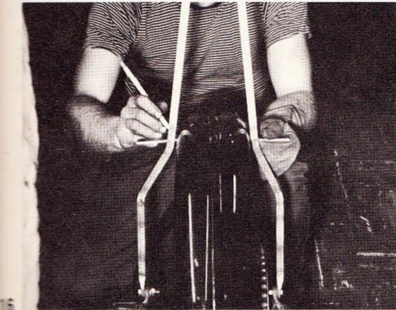
14 Bolt the ends of the bar to the fender brace mounting brackets, and once again check for straightness.
