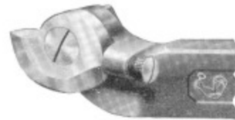
Fig. 11. Formed threading tool, solid type.
