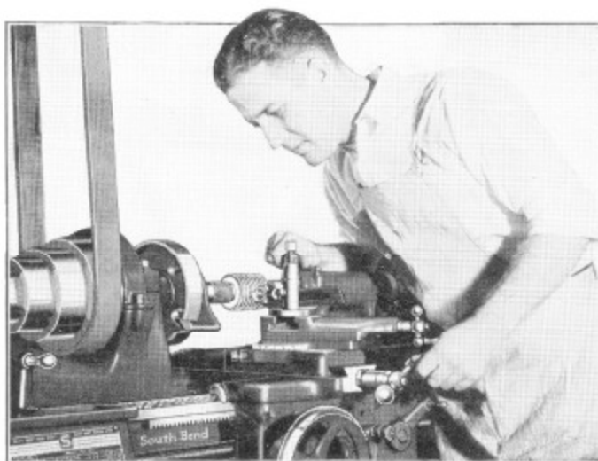
Fig. 1. Cutting a Screw Thread in the Lathe.
