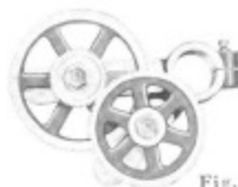
Fig. 42. Metric Transposing Gear Attachment for 16" Lathe.
